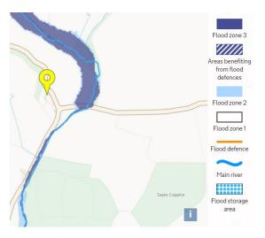
Golden Brook runs through the site (which is to the south west of the road junction at left). As can be seen from the EA flood mapping, the access road is subject to heavy flooding. After periods of heavy rain it becomes impassable to cars (this has happened frequently this winter). Additionally, Travellers' accommodation might be affected if sited close to the Brook.
